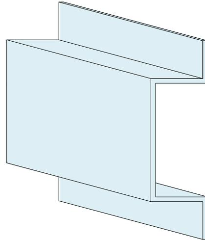
**FEDDERLITE CHANNEL SECTION VIEW**
